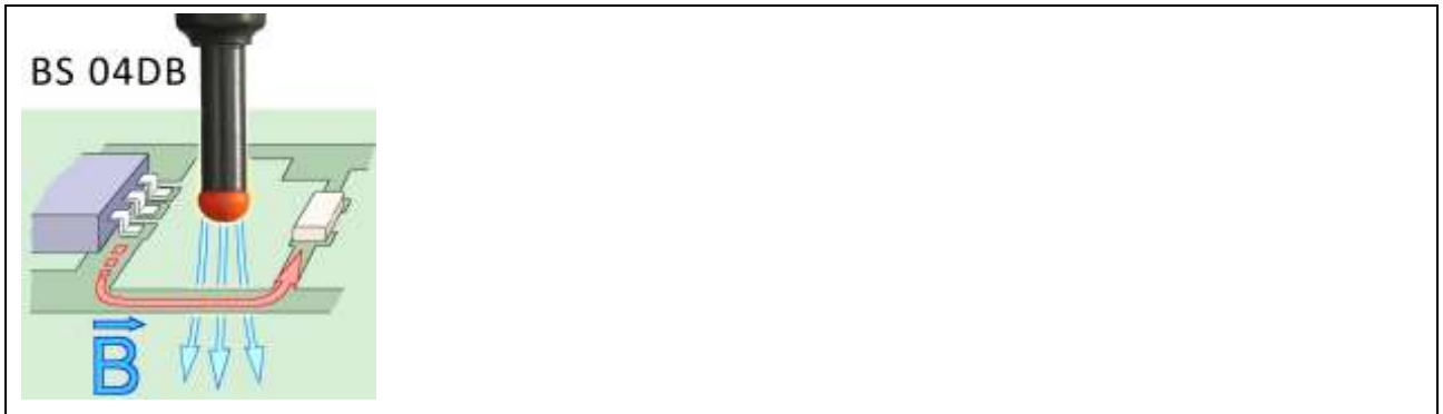
Figure 33: The magnetic field of the field source penetrates the conductor loop. and induces a voltage.
