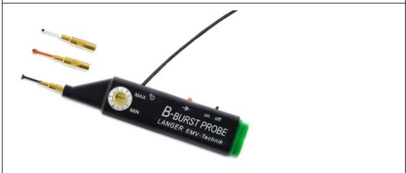
Figure 48: Magnetic field probe with exchangeable heads and an optical fibre from the S2 set.
