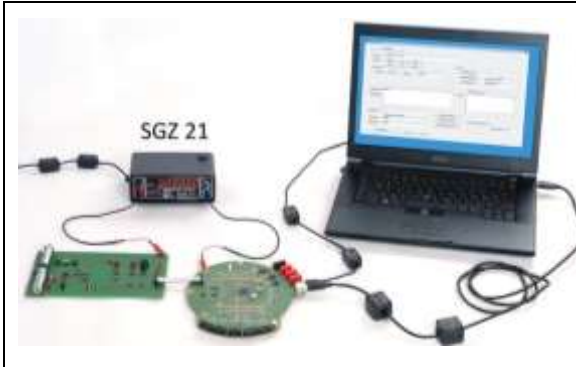
Figure 27: Injection of disturbance current via a two-pole connection and the connector of two modules. Contact is made to ground of each of the modules.
