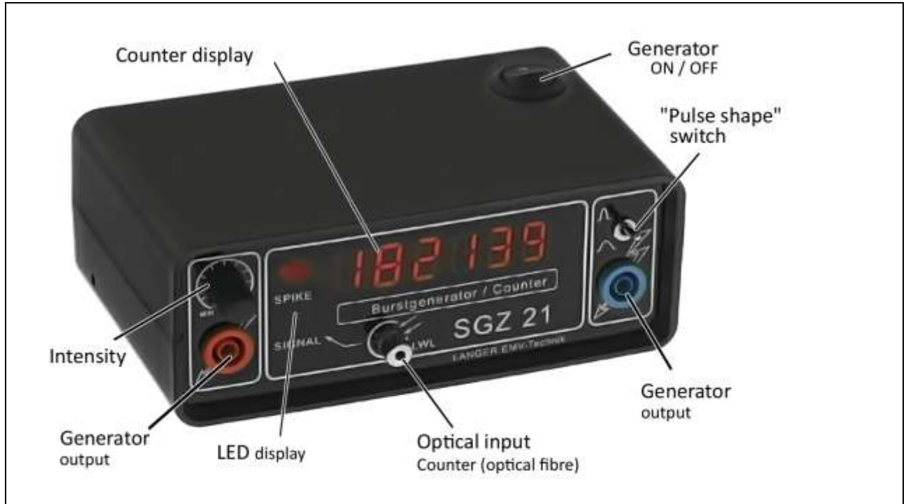
Figure 2: SGZ 21 pulse density counter / burst generator
