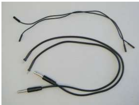
Figure 3: Generator cables (bottom); two extension cables (top).
