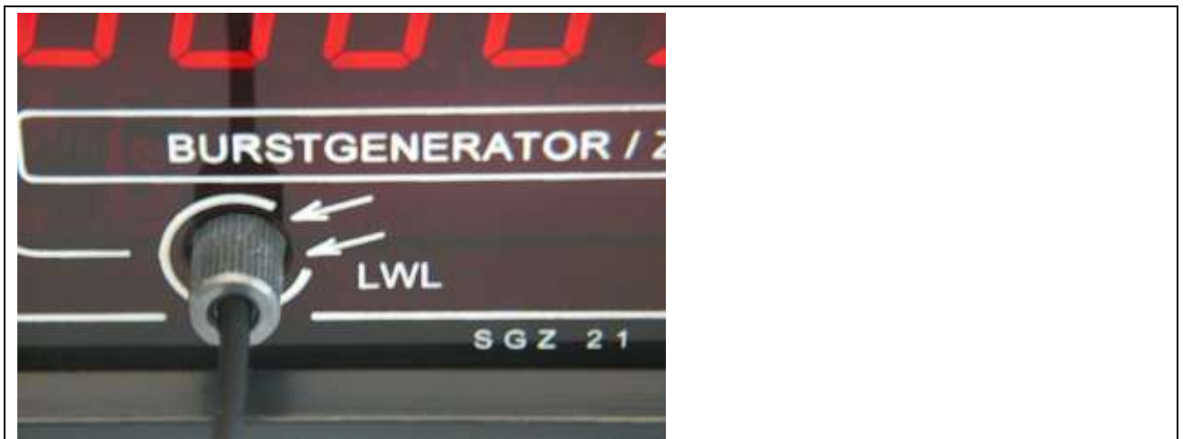
Figure 6: Optical fibre connection on the SGZ 21.
