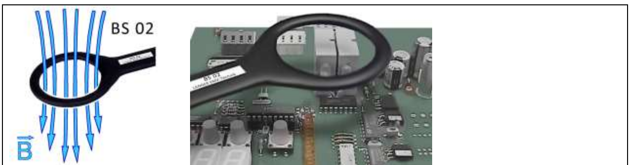
Figure 36: BS 02 field source with a large field beam to apply a magnetic field to conductor loops of around 10 cm.
