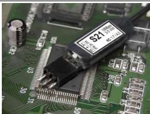
Figure 9: S21 sensor connected to an IC in the device under test, for example, via a three-pole socket.
